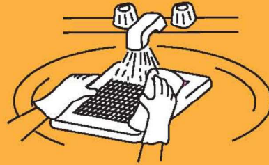
2. Wash and clean louver.
